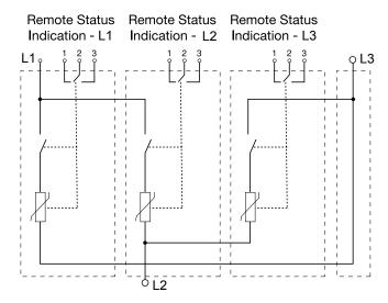
Wire Gage for Power - 25mm² (solid) 4AWG, 16mm² (flexible) 6AWG Wire Gage Remote Status Contact -  $6mm^2$  - 10AWG
